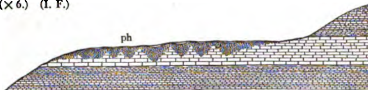
FIG. 1113. — Section in central Tennessee, showing the Upper Ordovician limestones with weathered surfaces, the product of weathering (chiefly the residual shells of Cyclora minuta , Fig. 1112, left on solution of the rock), accumulating in depressions and forming the phosphate rock (ph). The weathered phosphate-bearing surface is covered by late Palæozoic black shale, in the lower part of which some phosphate beds also occur. (After Hayes and Ulrich, Columbia folio, U. S. G. S.)
